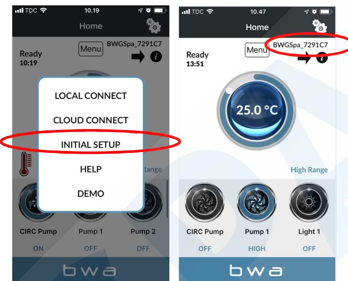
Second step is to connect your wifi module to your local wifi router in settings in the bwa app via the settings wheel. It has to be 2.4GHz and not 5GHz. You need to stay by your spa and have a good wifi range. Enter Network name and password and push below. As a standard the setup is set to WPA. You might need to choose WEP; WPS; OPEN, depending on your router.
